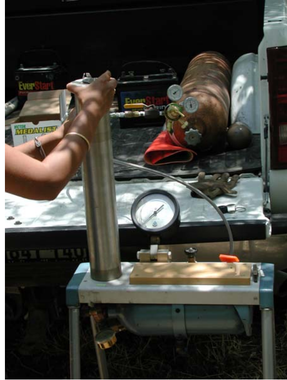
Pressure chambers were utilized to measure predawn and midday water potential of pecan leaves.
