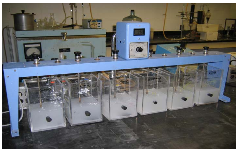
Figure 3. Laboratory Test Set-up for Conducting Lime Treatment Studies
